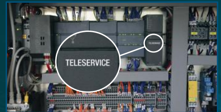
Possibility to remotely receive software updates on all the machine's electrical devices via teleservice
