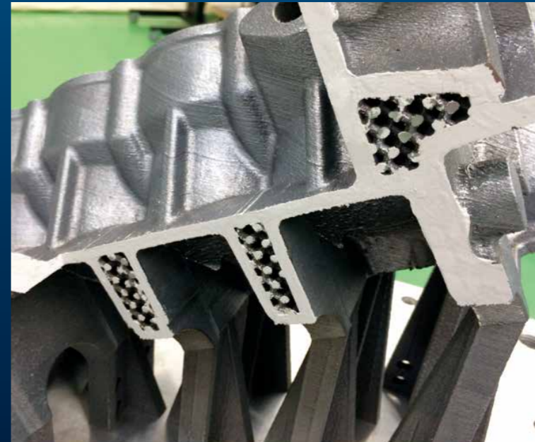
V8 engine block with lattice structure
